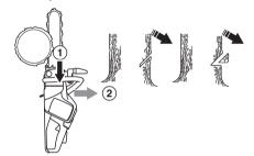
The directional cuts should run 1/4 of the diameter through the trunk and the angle between the top cut and bottom cut should be 45°.
