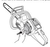
Press and hold the start button (>1 sec.) until the green LED is lit.
